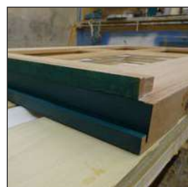
Seal top and bottoms of doors to prevent water from absorbing
