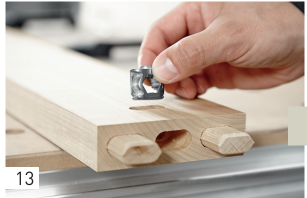
13 The cross anchor is then inserted into the cross mortise in the side wall, with the screw mortise facing upwards.
