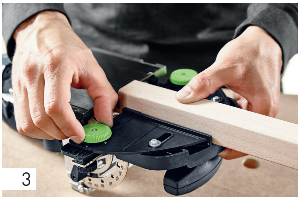
3 Using the spindle as a guide, ensure that the trim stop dimension fits perfectly; make further adjustments if necessary.
