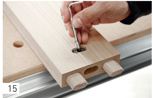
15 Then insert the threaded screw. Tighten it only so that the screw stays in place, but the opening remains open for the anchor bolt.
