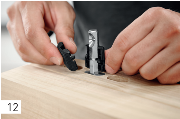
12 Clip the two DOMINO connector covers around the anchor bolt. These are used to hold the corner connector flush against the workpiece.
