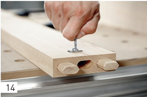
14 Press the cross anchor all the way into the mortise using the spanner.
