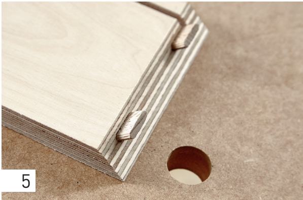
Insert the dominos into the mortises, glue them ...
