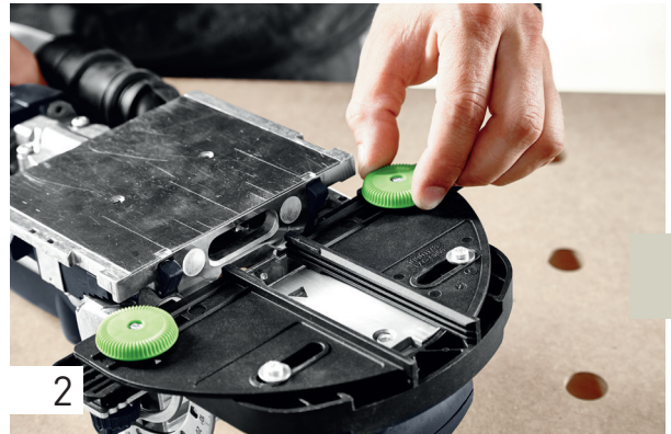
2 Set the width of the trim stop to the thickness of your spindle by adjusting the guide in the parallel side fence to the correct dimension using the scale and the green rotary wheels. In this example, we are working with 30 x 30 mm rectangular spindles.
