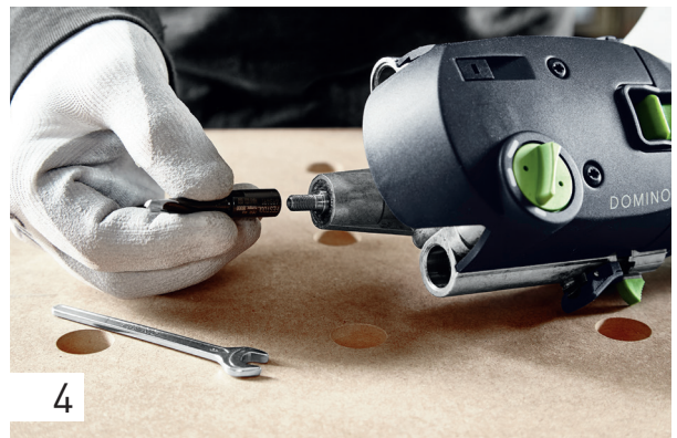
4 To process a 6 x 40 mm domino as in this example, use the 6 mm cutter (6 mm dominos can only be processed with the DF 500). For details on changing the router, see chapter 1.4.4, page 18.
