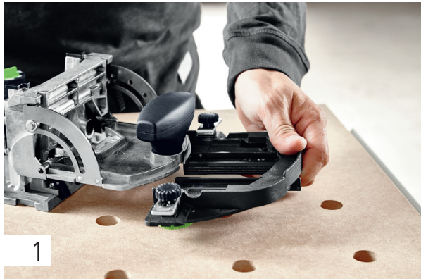
1 Mount the trim stop onto the DOMINO joining machine according to the operating instructions.
